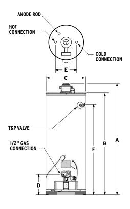
Maximum Hydrostatic Working Pressure: 150 PSI.
