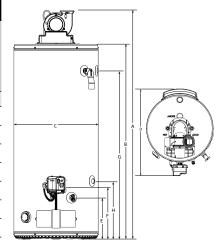
For propane models sub N for P. Natural gas models are series 200. Propane models are series 201.
