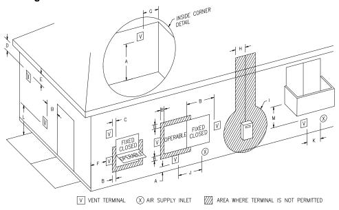
Figure 1 - Direct Vent Terminal Clearances
