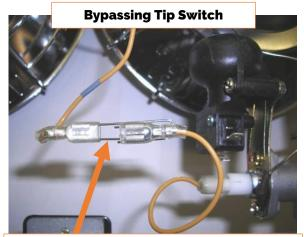
Use a paper clip to connect the two wire connectors together to bypass the tip switch.
