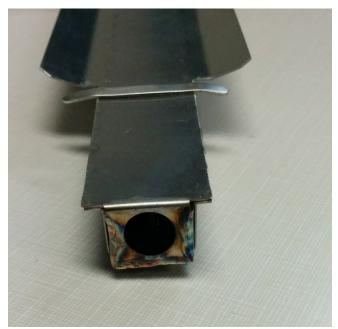
To ensure the burner is properly Seated, locate the orifice hole and the orifice (3). In the end of the burner there is an opening for the orifice to enter (2). Slide the burner opening onto the orifice (3) and secure to the burner bracket. NOTE: the burner will not align with the burner bracket if it is not properly seated onto the orifice
