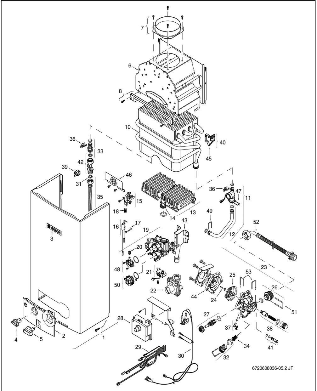
Fig. 27 Components Diagram
