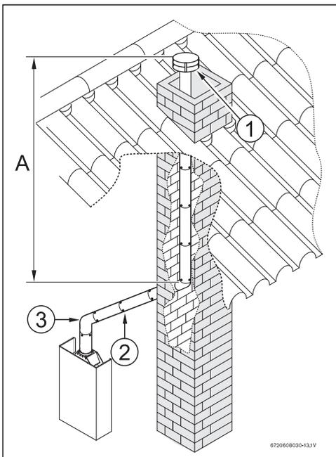
Fig. 12 Masonry chimney
