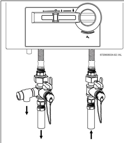
Fig. 15 Plumbing connections and pressure relief valve
