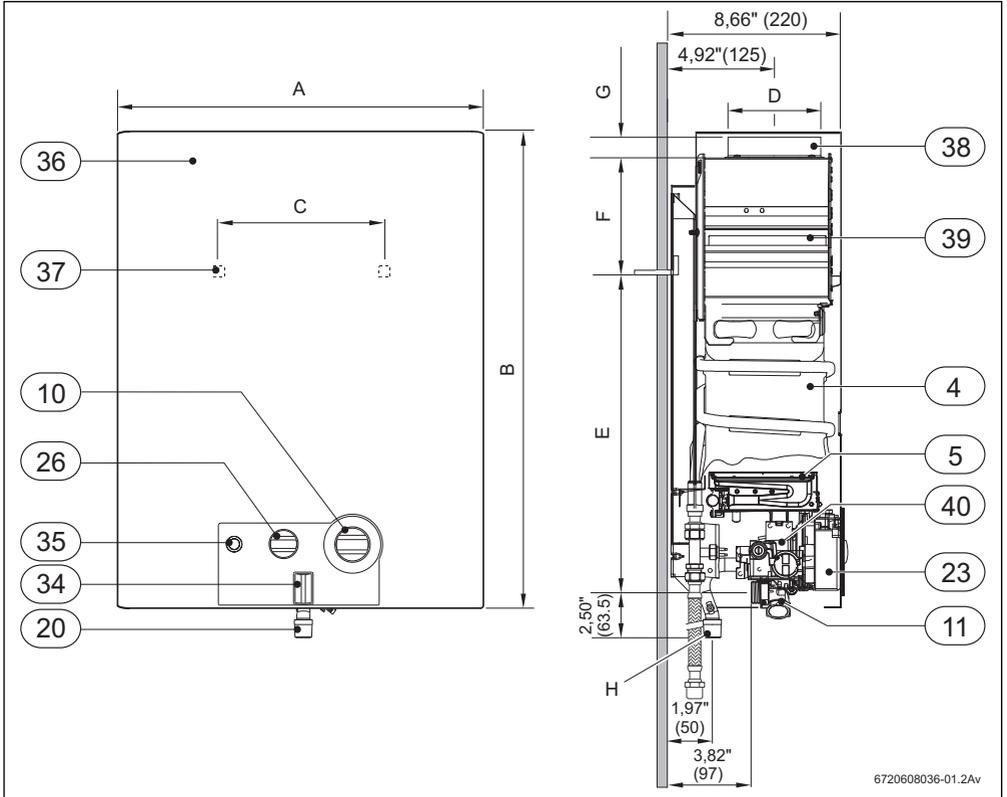
Fig. 3 Dimensions in Inches and (mm)
