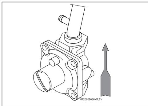
Fig. 13 Installation of Gas Pressure Regulator
